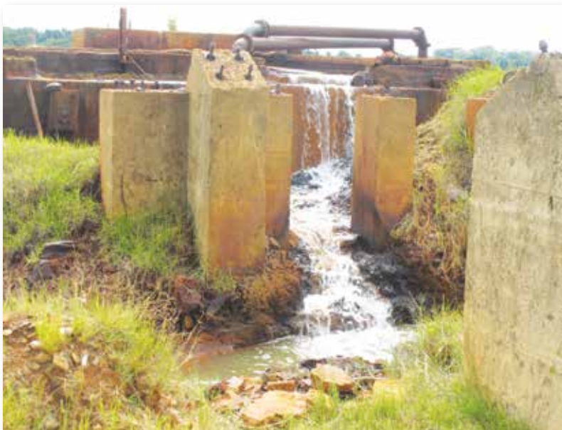
Picture 1: Illustration of decant of acid mine drainage taken from a mine shaft in the Wonderfontein catchment. Pumping prevents or at least mitigates against the risk of contamination of water found in the deeper mines.
