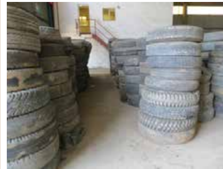
Photograph 3: Inadequate firebreaks between tyre stockpiles.
